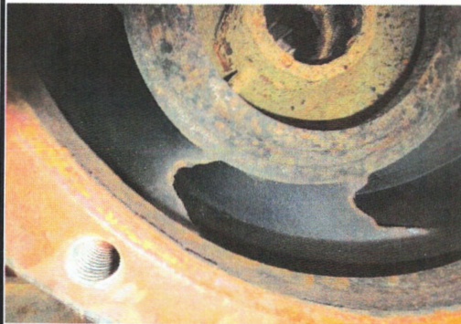
Excessive cutting of vanes
